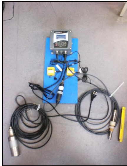
Figure 7 Solitex sc device with Turbidity probe (left) and EC probe (right).
