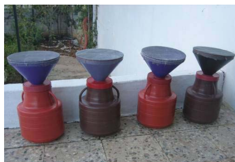
Figure 4.5b: Manual built supportive rain gauges for data accuracy.
