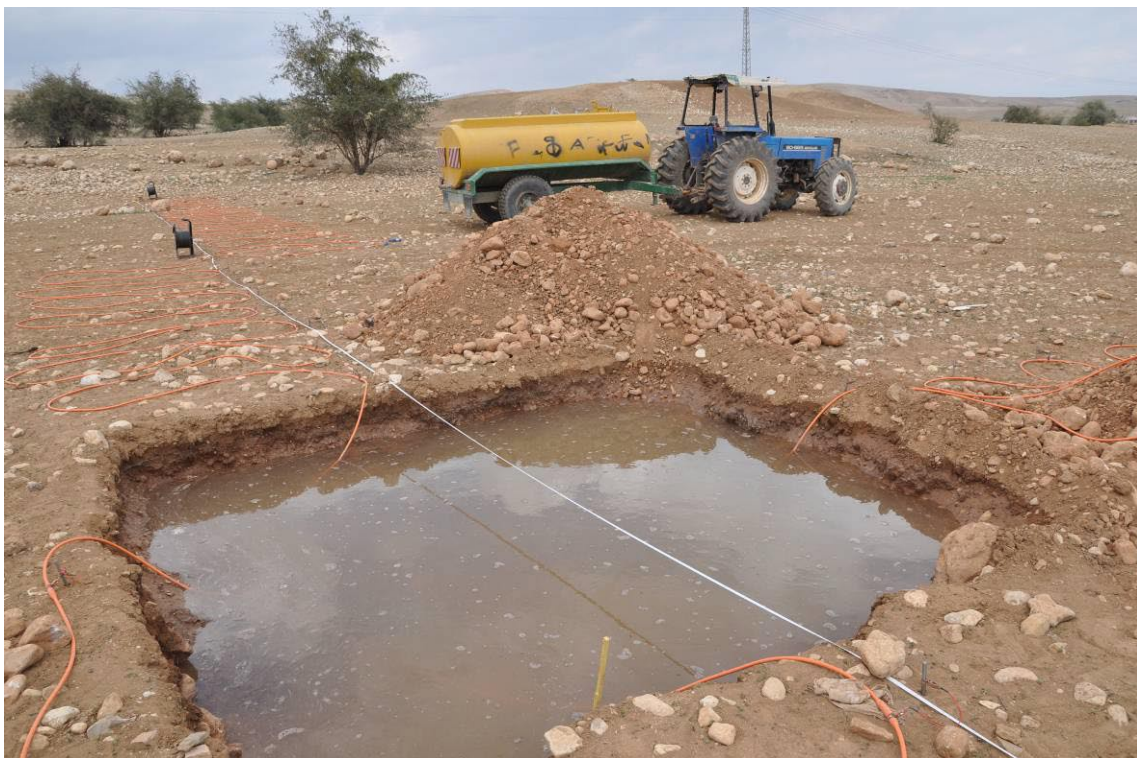
Figure 14: Pond filled with water for the infiltration experiment. Also the measurement device (orange cables and electrodes in the foreground) for the geoelectrical imaging can be seen.
