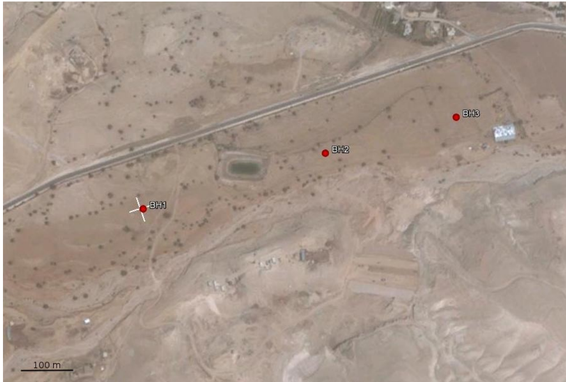
Figure 13: Location map of the geoelectrical arrays along the infiltration experiment (white cross). The infiltration basin is located in the centre of the cross. Also shown are the locations of the three exploration boreholes (Picture source: Google Earth).
