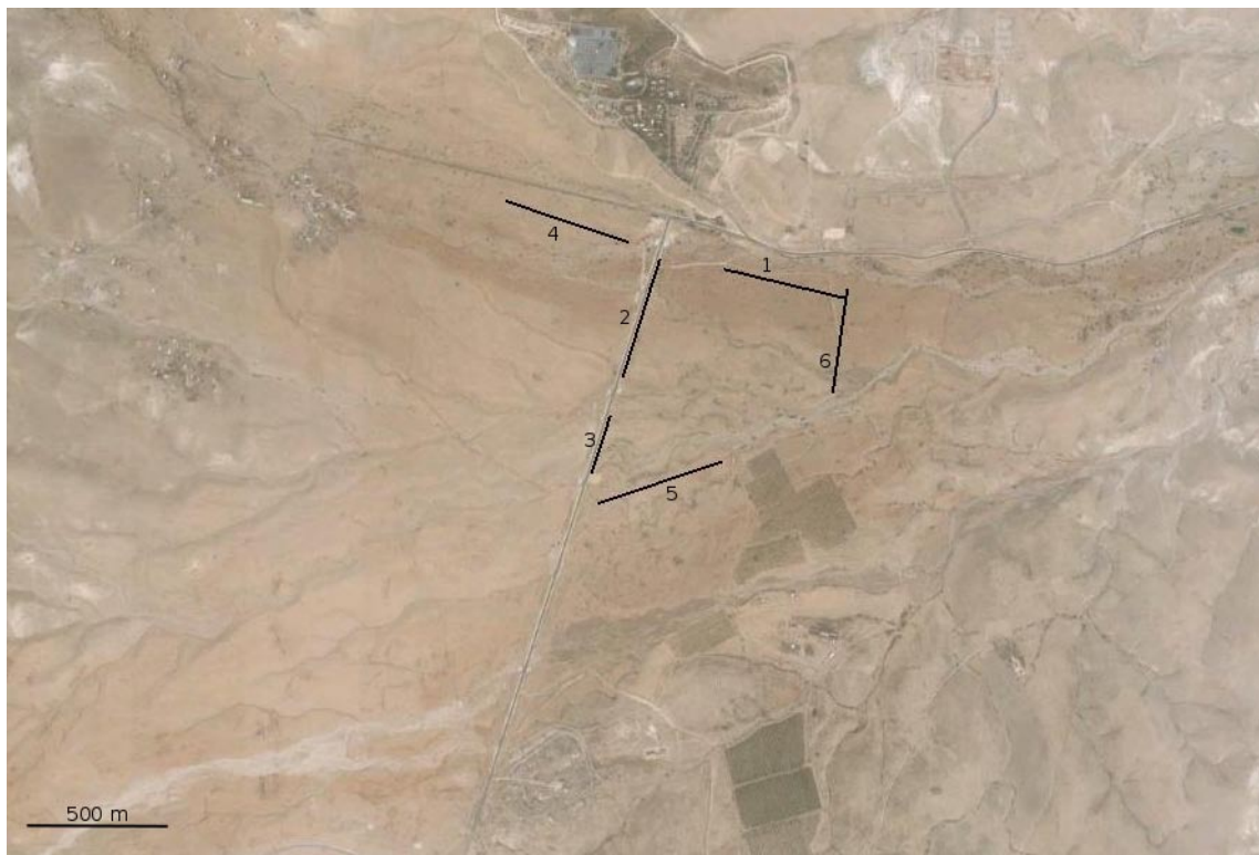
Figure 4: Location map of the refraction seismic arrays (Picture source: Google Earth).
