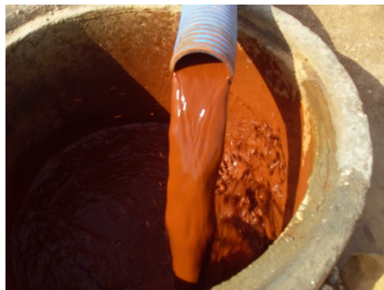
Figure 12: Well water after stop and restart of well pump (photo: SPA).
