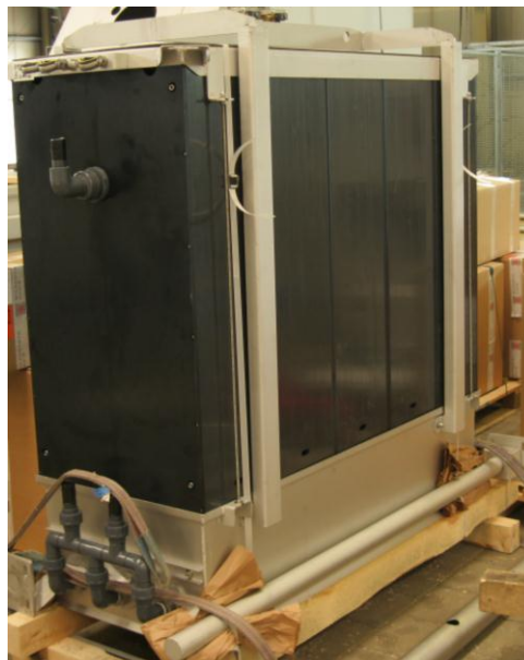
Figure 5: BioMem membrane module with adapters for scouring air and permeate withdrawal, during storage
